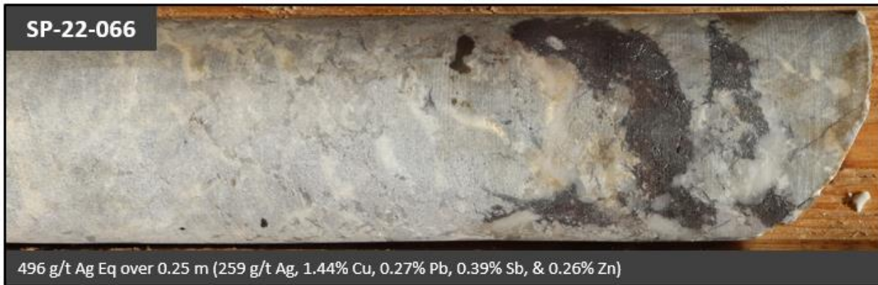
Figure 4: Dolostone-hosted breccia-style sulfide mineralization in hole SP-22-066 at 18.63 – 18.71 m
