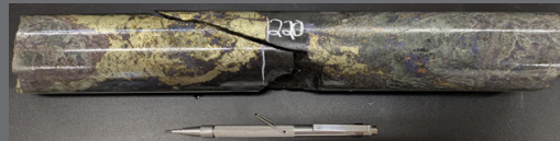
MEPS-25-02: 219.85 m, Bornite-chalcopryrite-gold, 23.1% Cu, 196 g/t Au, 168 g/t Ag over 0.6 m
