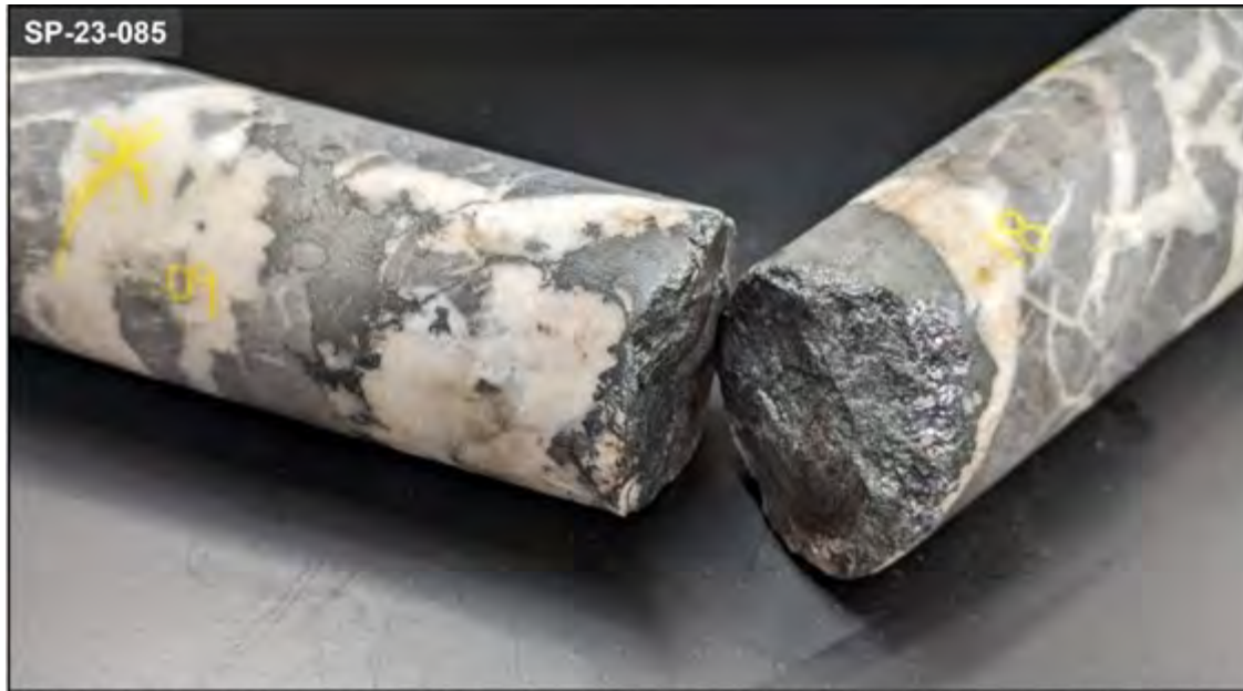
Figure 22: Drill core photo of high-grade mineralization in hole SP-23-085 from 208.97m to 209.29m.
