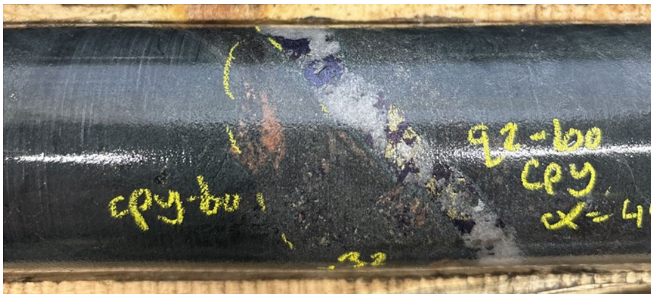
Figure 4. Bornite-chalcopyrite in quartz A-vein hosted by biotite-chlorite altered mafic volcanic adjacent to GFP porphyry dyke in hole MJ-25-02 at 245.3m grading 0.711% Cu, 0.11 g/t Au, and 9.4 g/t Ag.
