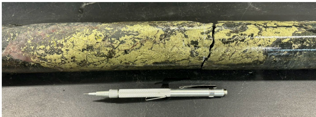
Figure 3. Massive Chalcopyrite-Magnetite mineralization at 157.7m depth grading 8.23% Cu, 1.28 g/t Au and 13.6 g/t Ag in hole CH-25-01. Host mafic volcanic is strongly biotite-altered with crosscutting quartz-orthoclase-hematite-magnetite-chalcopyrite “M”-veins.
