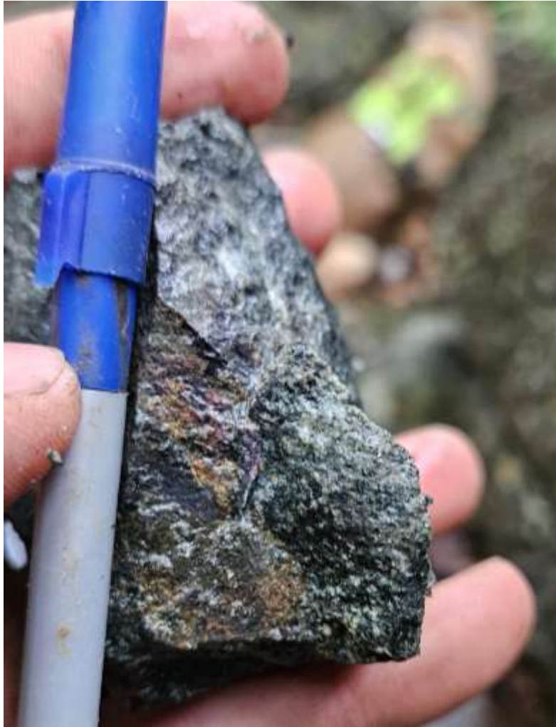
Figure 2. Bornite and chalcopyrite from grab sample SCFS-25-081 (assays pending) at Gimlet Target Area.
