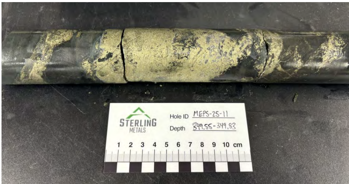
Figure 4. Massive chalcopyrite mineralization in MEPS-25-11 at 349.55m grading 13.1% Cu, 0.2 g/t Au, 22 g/t Ag and 340 ppm Mo
