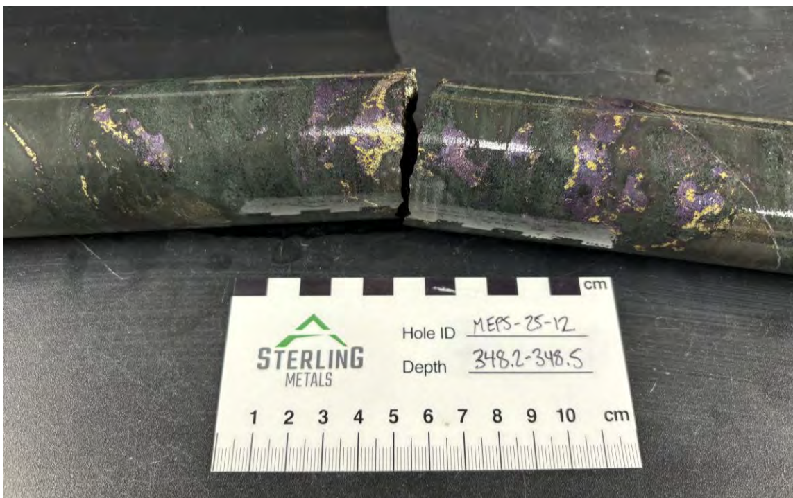
Figure 5. Bornite and chalcopyrite mineralization in MEPS-25-12 at 348.2m grading 8.2% Cu, 4.86 g/t Au, 71.4 g/t Ag and 20 ppm Mo
