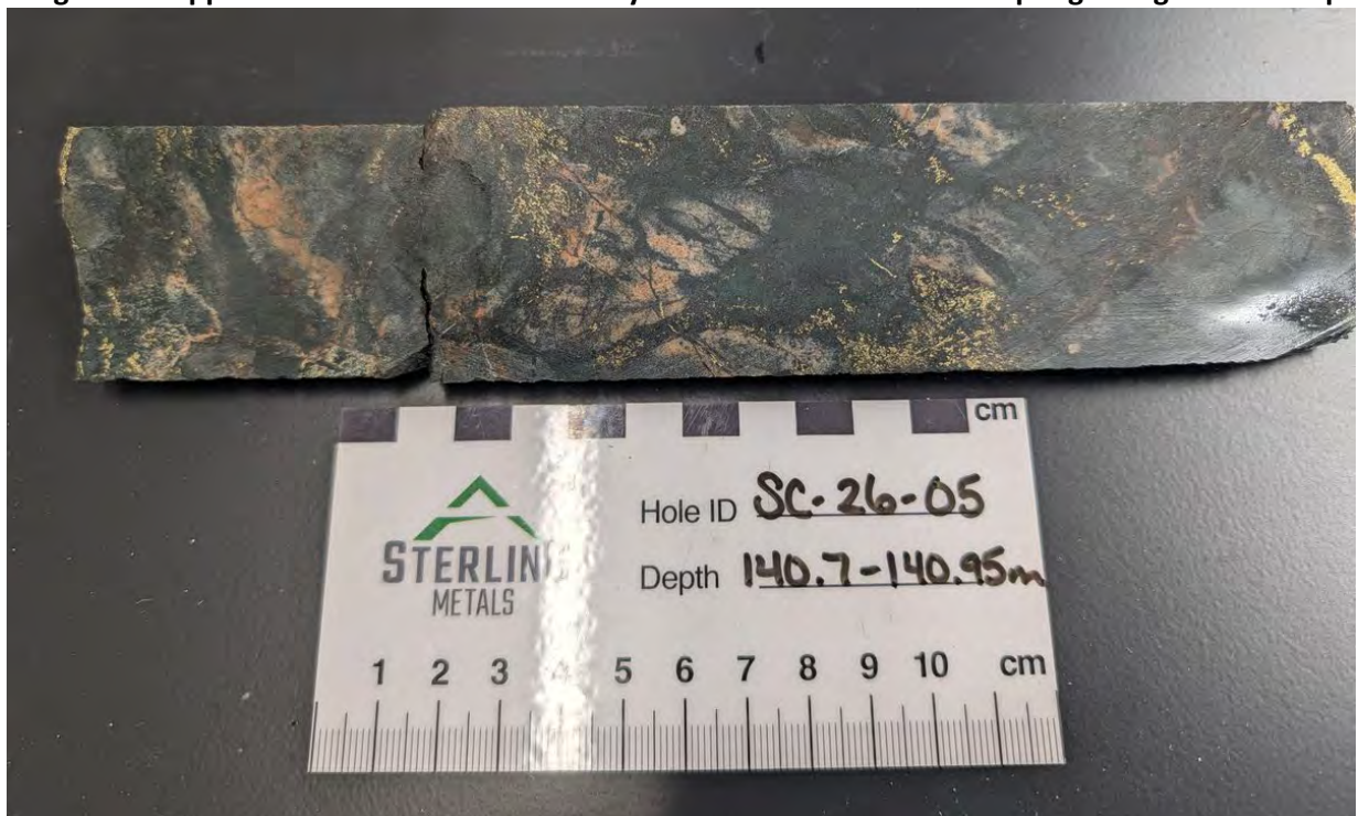
Figure 3. Copper mineralization above GFP dyke in SC-26-05 at 140.7m depth grading 1.79% CuEq
