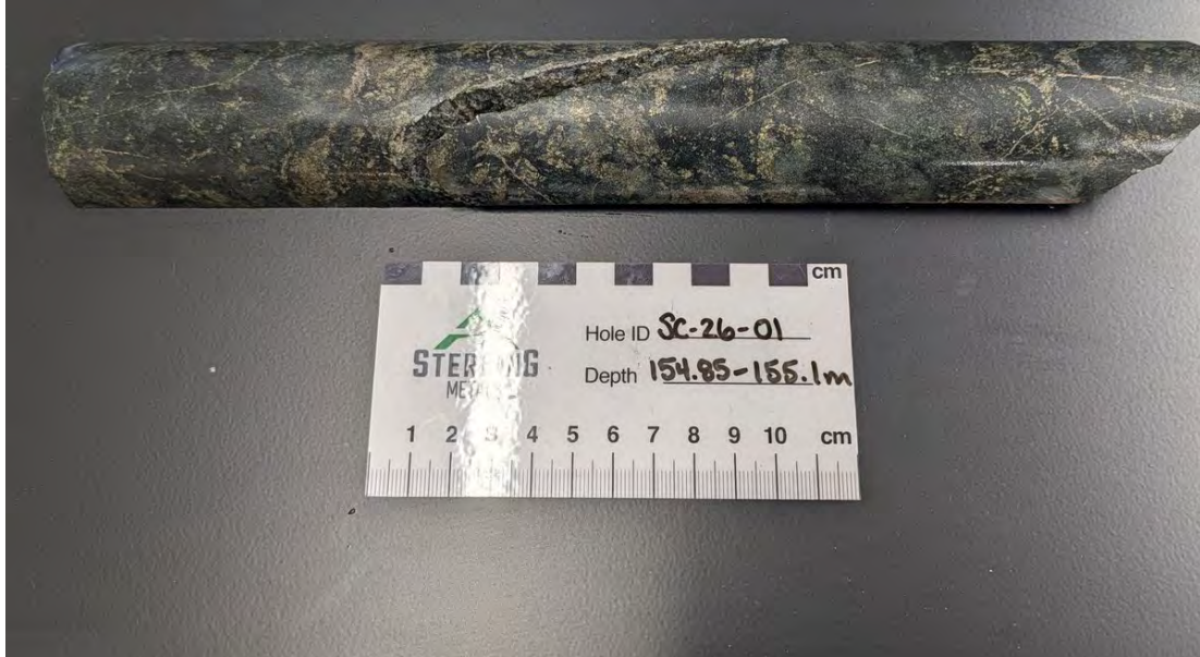
Figure 4. High-grade copper mineralization grading 2.07% CuEq in hole SC-26-01 at 154.85m depth, located approximately 1km east of the main MEPS discovery
