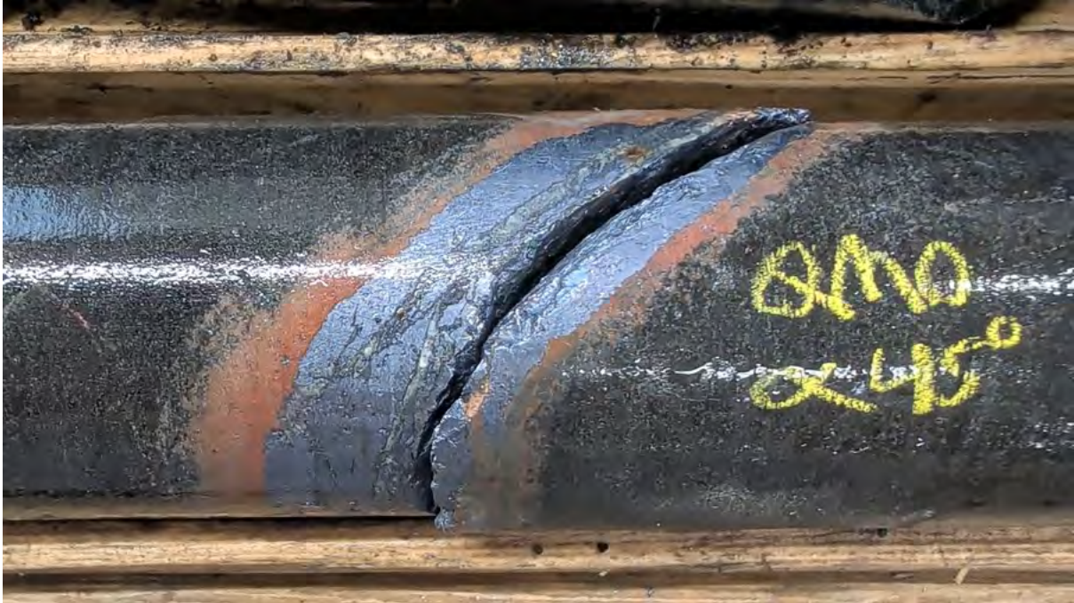
Figure 2. High-grade molybdenite core photo from hole SC-26-04 at 360.3m depth grading 1.7% Mo over 1m length
