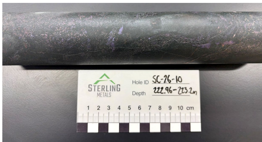
Figure 5. Example of mineralized core from SC-26-10 at 222.96 m depth grading 11.42% CuEq (9.56% Cu, 51 ppm Mo, 1.07 g/t Au, 80.6 g/t Ag).
