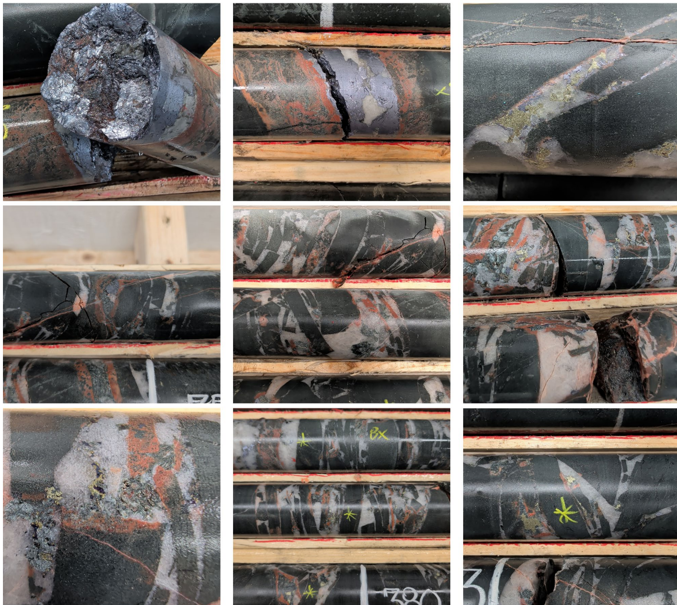
Figure 6: Core photos from the high-grade molybdenum zone highlighting very coarse-grained molybdenite-rich veins and a hydrothermal quartz shingle breccia hosting molybdenite, chalcopyrite and trace bornite.
