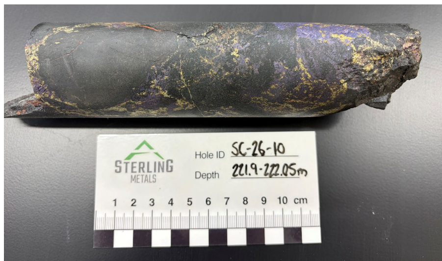
Figure 4. Example of mineralized core from SC-26-10 at 221.90 m depth grading 8.83% CuEq (7.58% Cu, 166 ppm Mo, 0.56 g/t Au, 62 g/t Ag).
