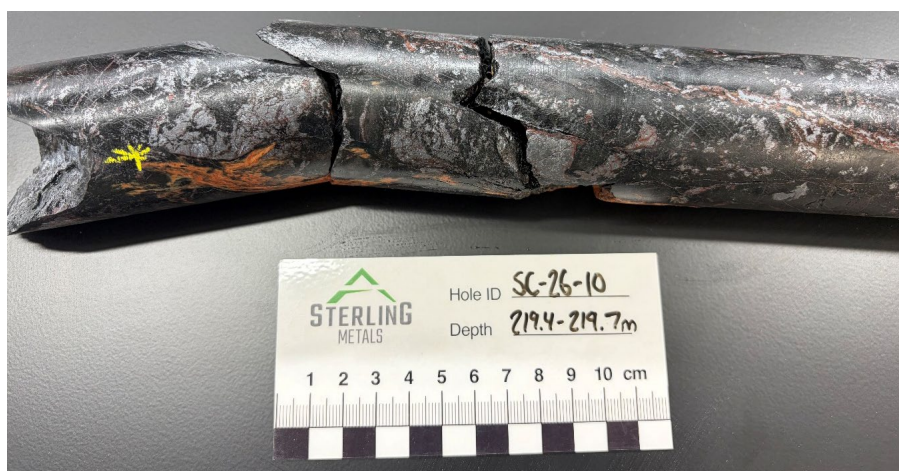
Figure 3. Example of mineralized core from SC-26-10 at 219.40 m depth grading 8.08% CuEq (6.55% Cu, 52 ppm Mo, 0.99 g/t Au, 57.1 g/t Ag)
