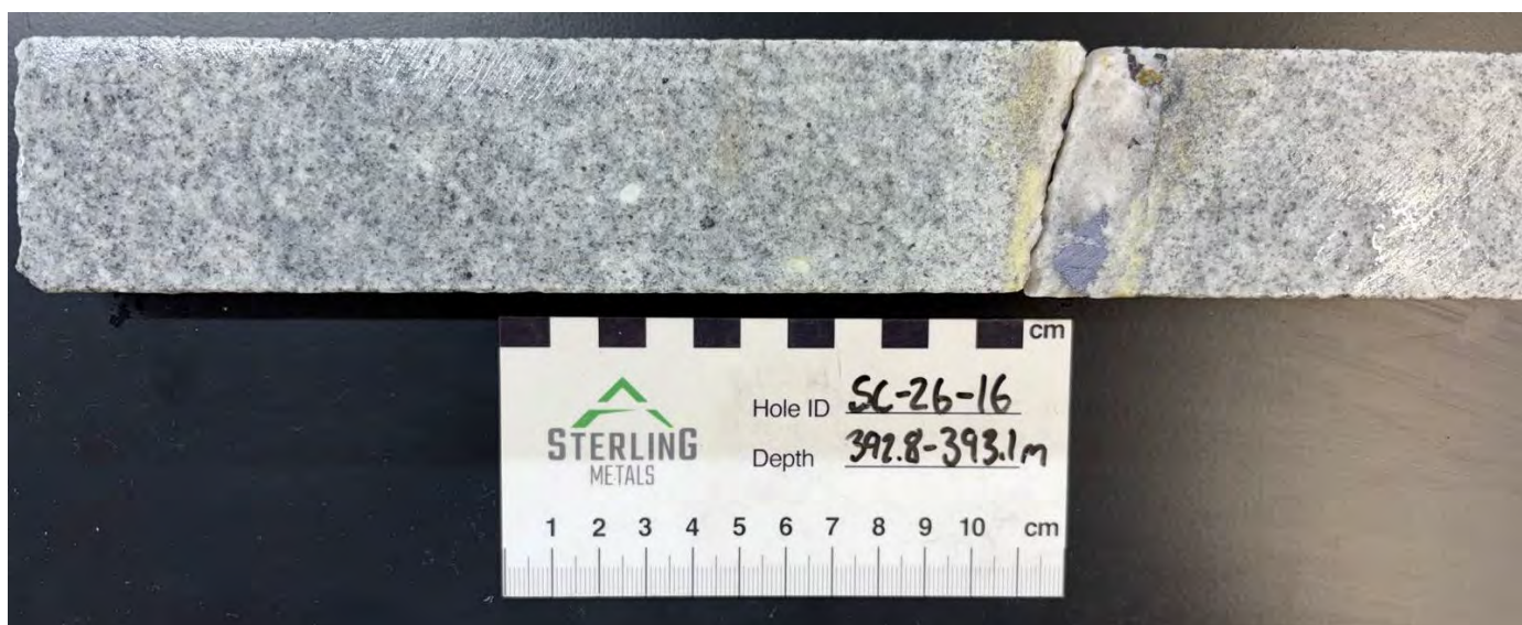
Figure 4. Representative core photograph from SC-26-16 showing typical molybdenite-rich quartz-sericite vein within mineralized granite porphyry stock at 392.8m depth grading 0.024% Cu, 0.0025 g/t Au, 1.9 g/t Ag, 1.6% Mo (8.21% CuEq)
