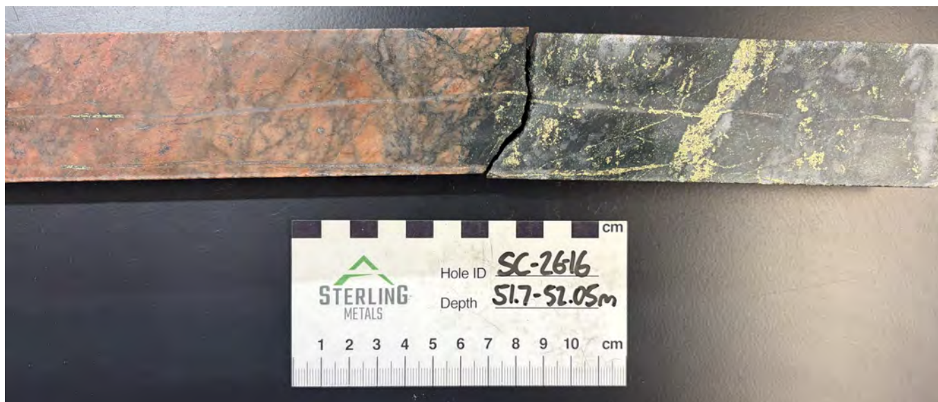
Figure 3. Representative core photographs of GFP unit and copper mineralized ribbon vein below with associated higher copper grades at 51.7m depth grading 4.21%Cu, 0.23 g/t Au, 18.3 g/t Ag and 11ppm Mo (4.62% CuEq).
