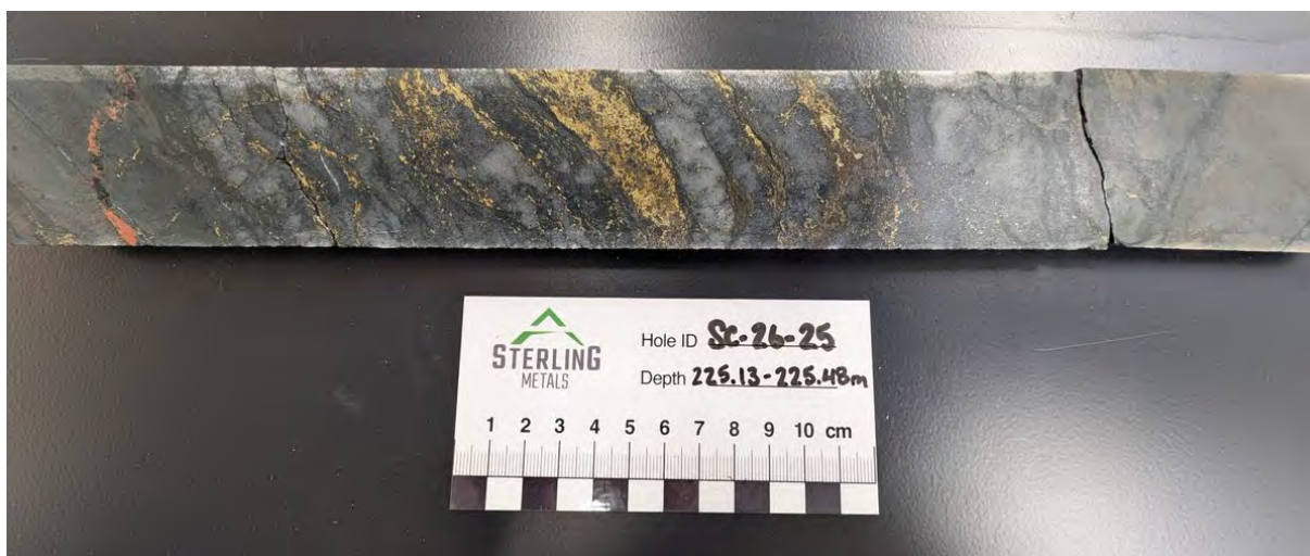
Figure 6. Ribbon vein with copper sulphides in hole SC-26-25 from 225.13m to 225.48m depth grading 2.71% CuEq (2.52% Cu, 0.113 g/t Au, 8 g/t Ag, 5ppm Mo)
