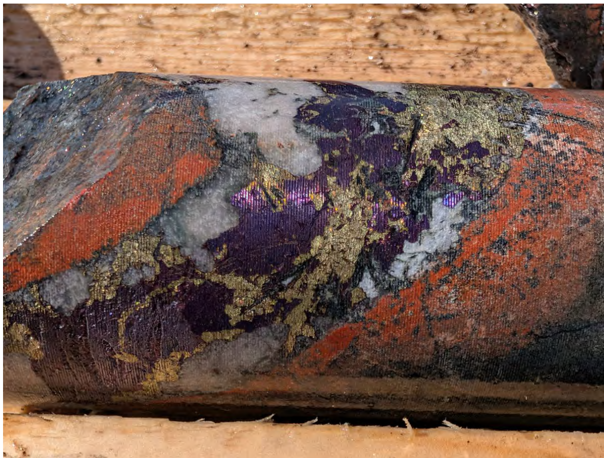
Figure 3. Copper-gold rich vein containing bornite (purple) and chalcopyrite (yellow) in hole SC-26-26 from 293.62m depth grading 6.02% CuEq (2.17% Cu, 3.92 g/t Au, 27.8 g/t Ag, 2 ppm Mo)
