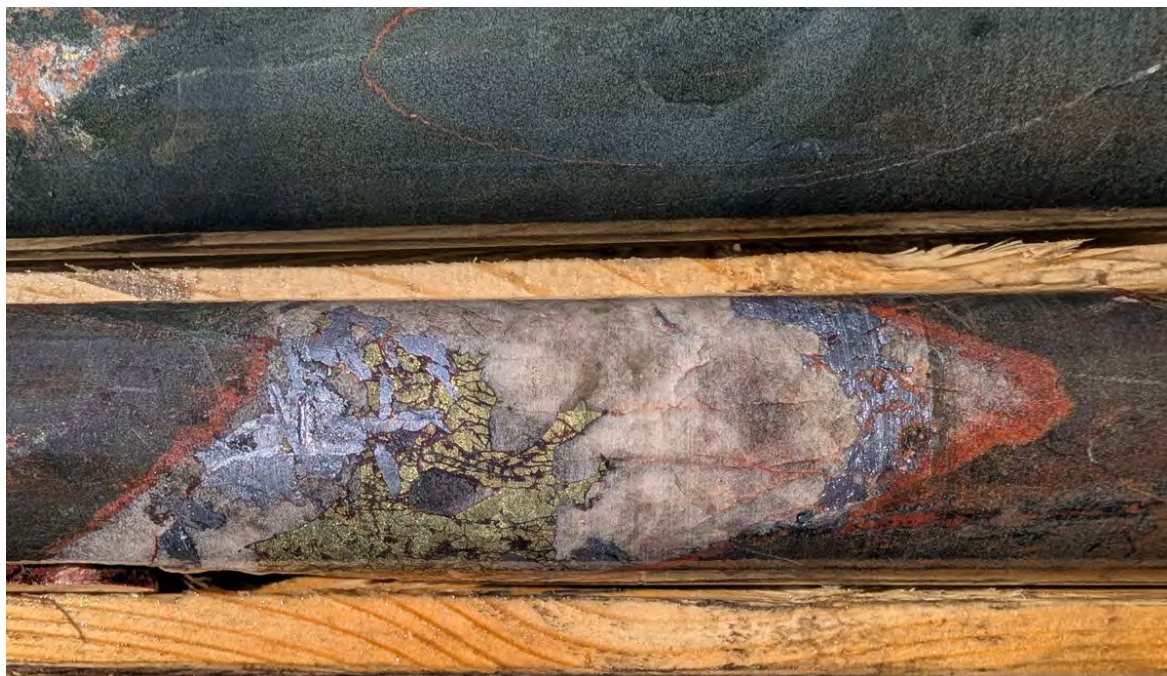
Figure 4. Copper sulphides (chalcopyrite and bornite) and molybdenite (silver grey mineral) in quartz vein hosted by biotite-magnetite altered basalt in hole SC-26-26 from 282.5m depth grading 10.53% CuEq (2.56%Cu, 0.265g/t Au, 12.5 gpt Ag, 14900 ppm Mo)
