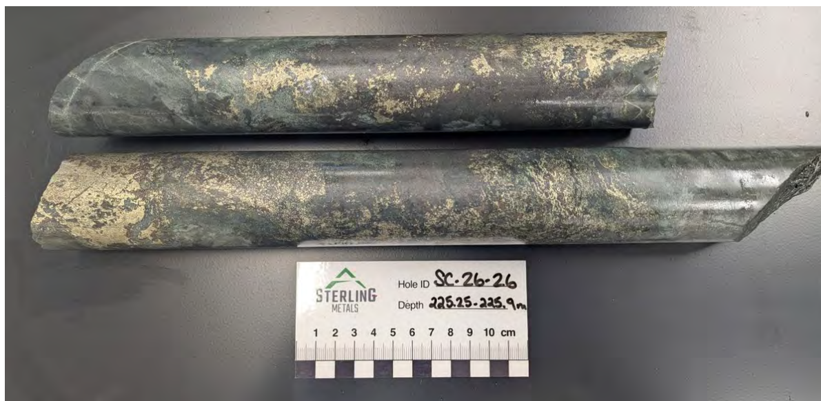
Figure 5. Copper sulphides (chalcopyrite) hosted within potassic-altered (biotite-magnetite) basalt in hole SC-26-26 from 225.25m depth grading 5.08% CuEq (4.68%Cu, 0.175g/t Au, 12.2 g/t Ag, 123ppm Mo)
