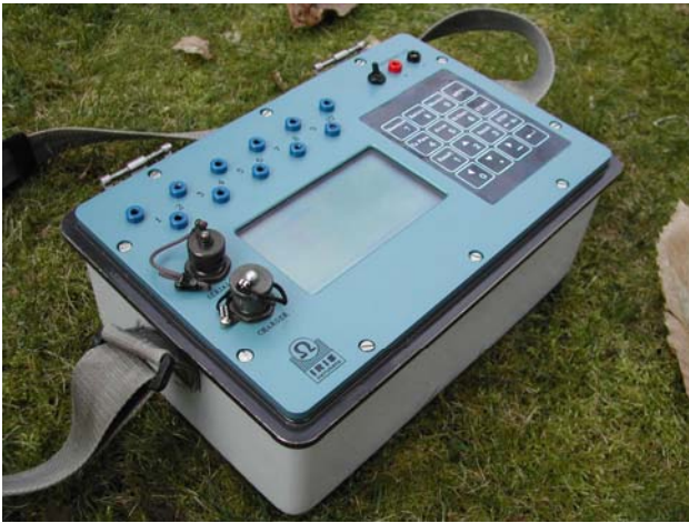
ELREC Pro unit with its graphic LCD screen
