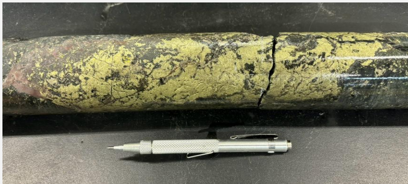
Massive Chalcopyrite-Magnetite mineralization at 157.7m depth grading 8.23% Cu, 1.28 g/t Au and 13.6 g/t Ag in hole CH-25-01. Host mafic volcanic is strongly biotite-altered with crosscutting quartz-orthoclase-hematite-magnetite-chalcopyrite "M"-veins.
